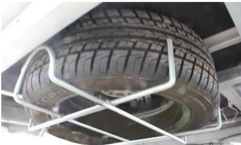
Unfortunately accidents do happen, but with the OPUS Spare Wheel and Carrier you can be prepared. The Carrier is a steel hinged retaining frame fixed to the underneath of your OPUS, and includes a spare wheel with tyre, based on your choice of wheel. So you can be confident that you are ready if for all eventualities.
